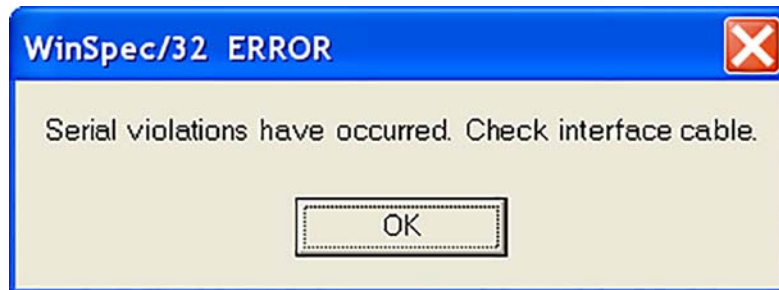
Figure 7-6: Typical Serial Violations Have Occurred Dialog
