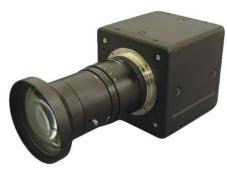
The BV-C3300 employs a special prism optics to separate P wave and S wave components and each image is captured by 4K line sensor respectively. The BV-C3300 outputs P wave image and S wave image at the same time. This is very effective for inspecting front and back of the transparent materials with thickness such as detecting scratches on the both sides of the glass, electric parts inspection on the board and contaminants inspection for raw materials.
